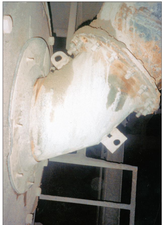
Left and right. The North Texas Cement inlet elbow transporting raw feed to the ball mill.
