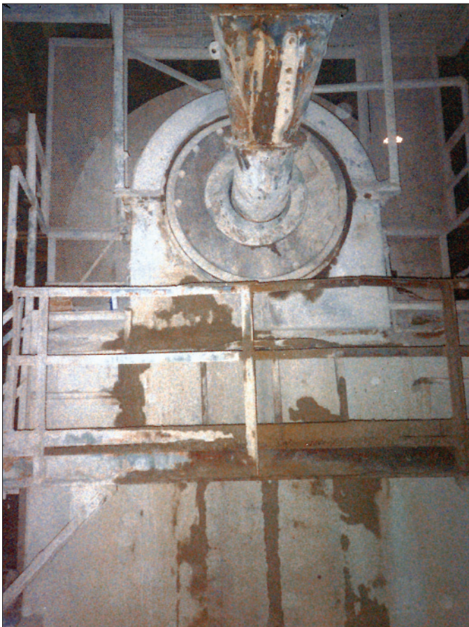
Left and right. The North Texas Cement inlet elbow transporting raw feed to the ball mill.
