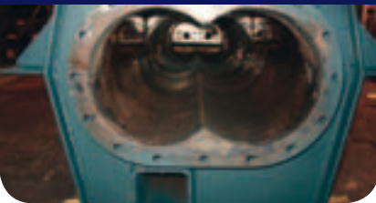
Figure 4: view through the dual-screw conveyor housing
